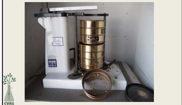
Rotap shaker showing 4.75mm screen and corn retained on the sieve
