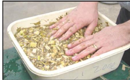
Figure 2. Gently agitating material to help the kernels sink to the bottom of the container.
