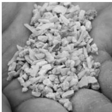
Figure 3: Struvite Crystals (Dangaran)
