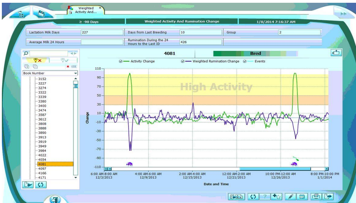
Figure 2: Graphic representation of an animal (cow ID 4081) with weighted activity and rumination data provided by the monitoring device.
