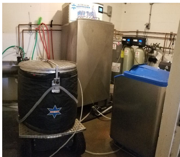
Figure 1. The HL Milk Taxi which pasteurizes and transports the milk (left), the Milk Jug cooling tank where milk is stored (middle), and the Holm & Laue HL100 Programmable Automatic Calf Feeder (right).
