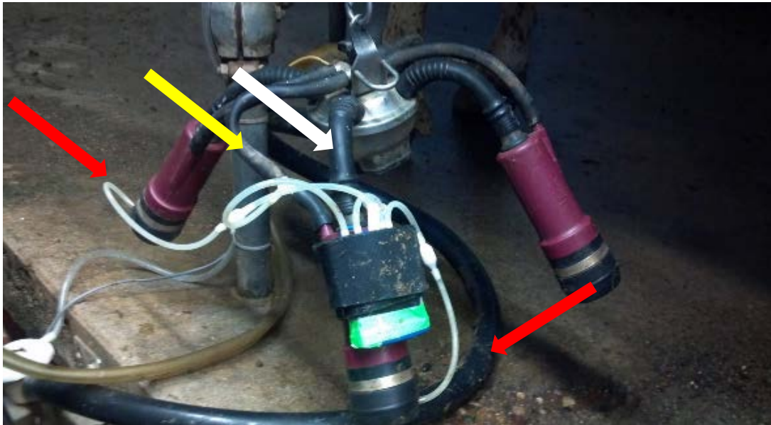
Figure 1: VaDia units measure vacuum in the mouthpiece of a front and rear liner (red arrows), near the cluster (short milk tube, white arrow) and in a short pulsation tube (yellow arrow).
