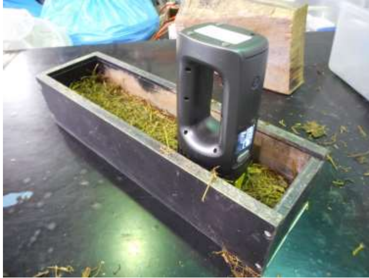
Figure 1: The Neo Spectra instrument and sample in preparation for scanning.
